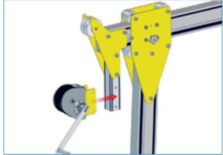
6. Place the winch and bracket in position.
