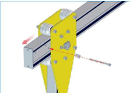
3. Insert and secure bolt and spacer as shown.
