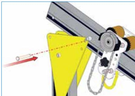
6. Present the beam to the column and insert clevis pin to take the weight of the beam
