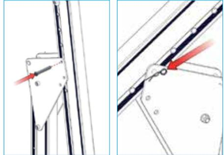
5. Present the beam to the chosen location and insert the clevis pin. **Secure the pin with retaining R-clip.**
