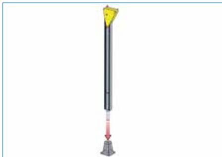
5. Insert T-DAVIT column into the socket
