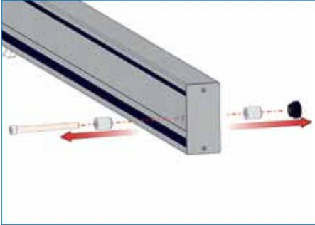
1. Remove bolt and spacer at the front of the beam
