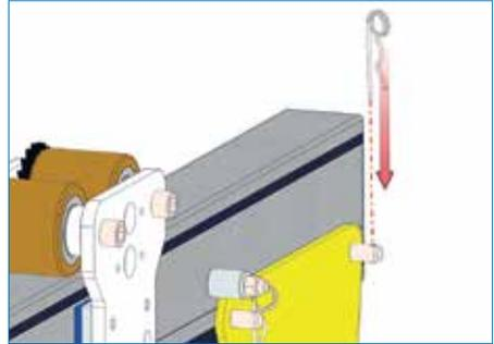
10. Secure the pin with retaining R-clip
