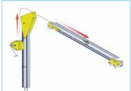
3. Play out sufficient rope to thread through the length of beam whilst at ground level. Thread the rope over the sheaves and through the beam as shown.
