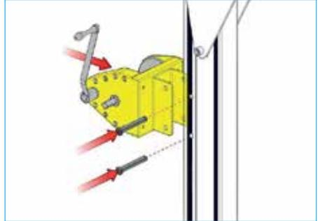
2. The T-DAVIT has the option to install a winch on the column as illustrated in the image. **Ensure the clevis pins are secured in place using the R-clips.**
