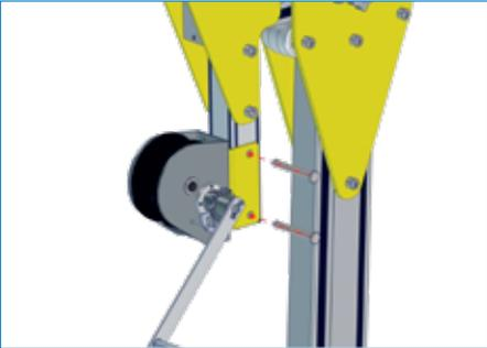
7. Secure assembly with the pins supplied.
