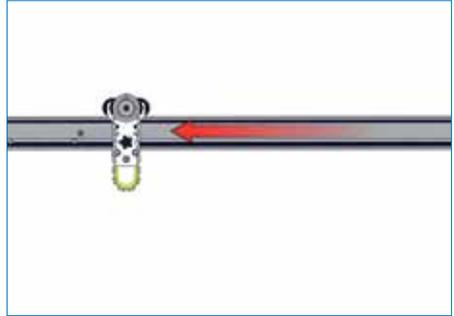
2. Thread beam trolley over the end of the beam
