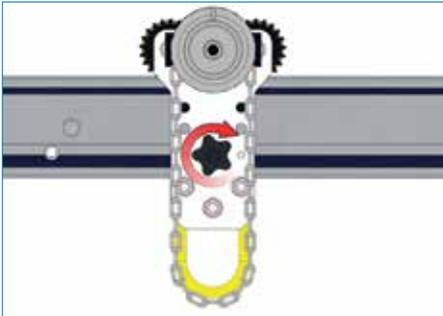
3. Lock trolley with friction brake at approximately centre position
