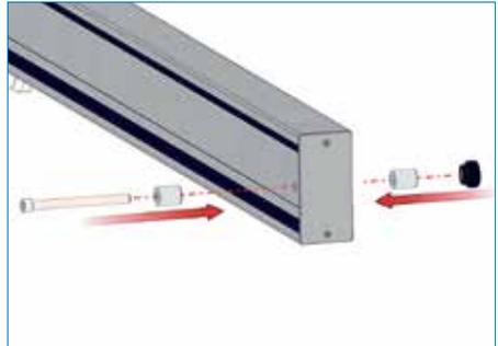
4. Reinsert bolt and spacer ensuring they are secure.
