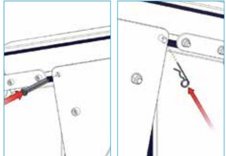
7. Insert the clevis pin to take the weight of the beam and **secure the pin with the R-clip.**
