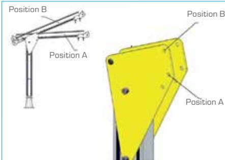
4. The T-DAVIT beam can be assembled at 2 positions as shown. Ensure the correct set-up is chosen at this stage.
