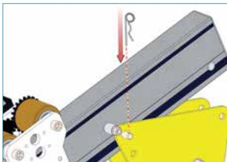
7. Secure the pin with retaining R-clip
