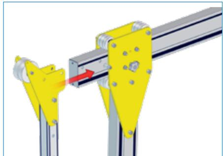
4. Place winch attachment column to the beam as shown.
