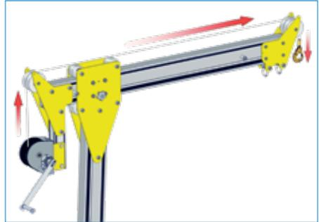
8. Thread the rope over the sheaves. The rope retaining pins need to be removed before fitting the rope.
