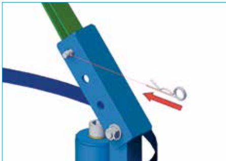
7. Insert retaining clip through adjustment pin.
