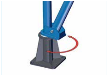
8. Check the davit assembly for ease of rotation.
