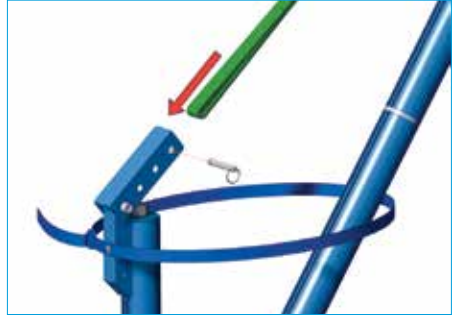
6. Supporting the weight of the jib with the shoulder, select required operating radius and attach tension strap to adjust channel with the adjustment pin.
