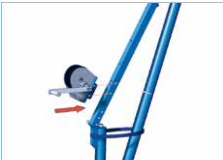
7. Position winch on rigid adjustment channel and attach winch with retaining pins and clips. Ensure winch rope is wound correctly.
