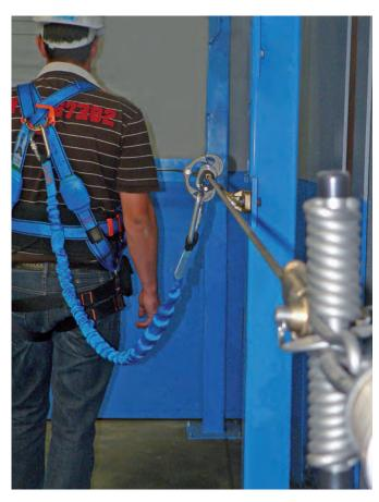
The Travsmart lifeline complies with the requirements of the EN 795 C standard and can be used simultaneously by 5 users. The intermediate supports must be located at 15 metres. The Travsmart lifeline can be installed under a ceiling, on a wall, on an inclined surface up to 5°, on the ground or on a post.
