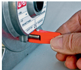
➤ Disengageable drum, no load only.
