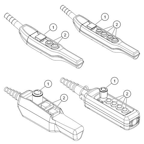
Figure 9. Examples of pendant controller types
