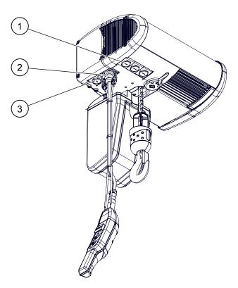
Figure 7. Cable gland positions of the chain hoist
