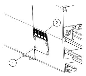
Figure 32. Location of the cover plate and adjustment sticker of the GLS on the hoist profile
