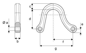
Figure 12. Dimensions of the suspension bracket
