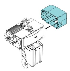
Figure 36. Chain hoist with extension profile
