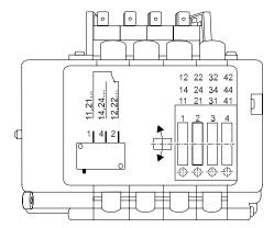
Figure 35. 4-step rotating geared limit switch
