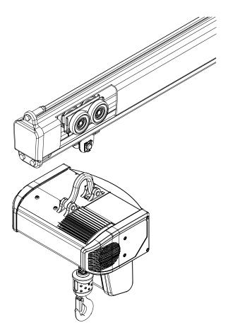
Figure 39. Push trolley inside LCS profile
