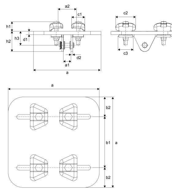
Figure 15. Dimensions of the fixed suspension
