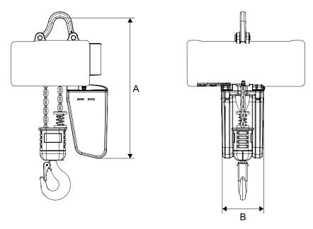
Figure 19. Chain bucket dimensions
