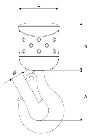
Figure 26. Dimensions of the single fall hook block
