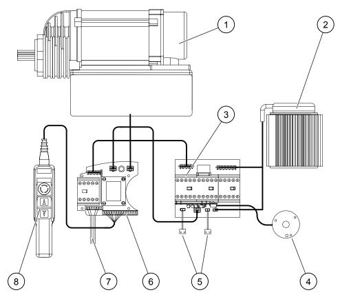
Figure 8. Wiring principle of the electrical chain hoist
