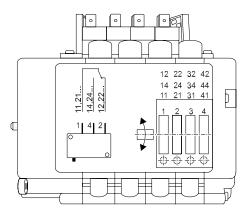
Figure 31. 4-step rotating geared limit switch
