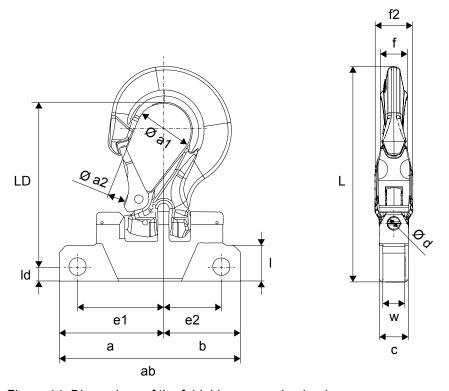
Figure 14. Dimensions of the foldable suspension hook
