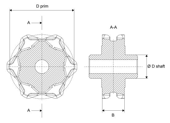
Figure 17. Dimensions of the return sprocket
