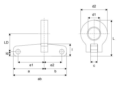
Figure 13. Dimensions of the suspension eye
