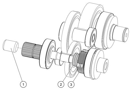
Figure 6. Slipping clutch construction with one clutch disc
