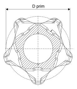
Figure 16. Dimensions of the chain sprocket
