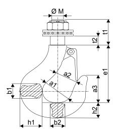
Figure 20. Dimensions of the standard hook
