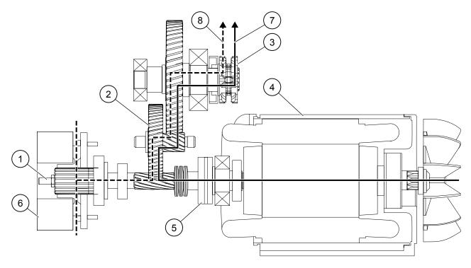
Figure 3. Kinematic chain of the electrical chain hoist
