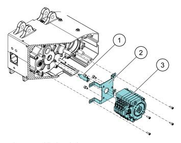
Figure 29. 4-step rotating geared limit switch
