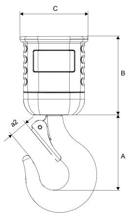
Figure 28. Dimensions of the two-fall hook block
