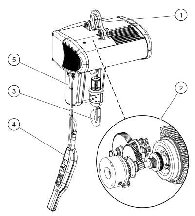
Figure 1. Main components of the electrical chain hoist
