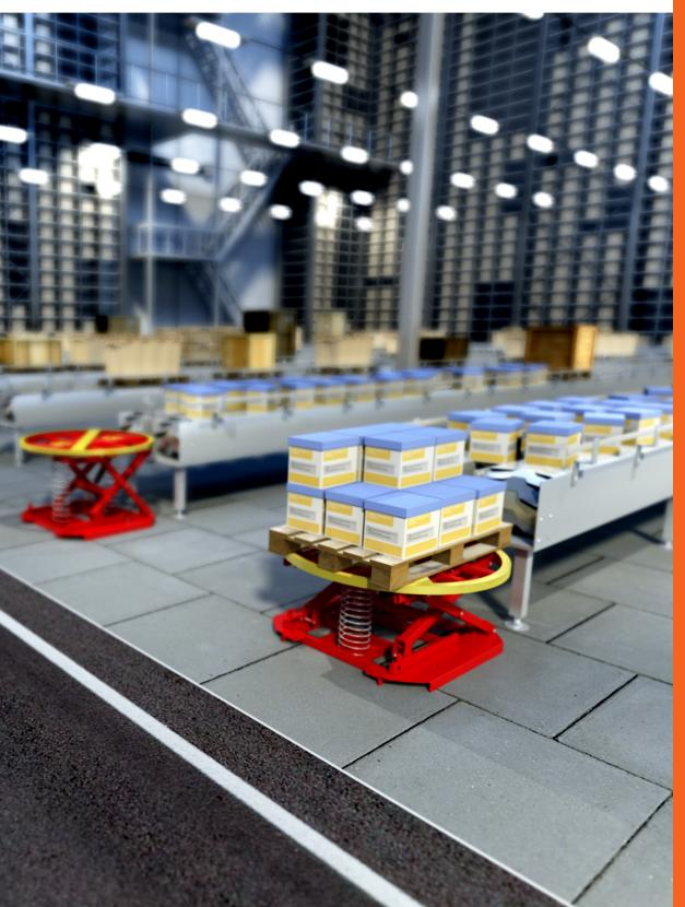
Spring Level Loaders automatically adjust the height of pallet loads as boxes are added or removed. eliminating bending, reaching and stretching. With loads kept at a constant height, workers can build and break down pallet loads quickly and easily, with minimum effort and risk of injury. A built-in turntable top allows workers to spin the load so they can remain in one spot throughout the loading and unloading process.
