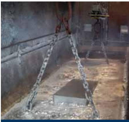
Addition of zinc blocks
